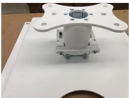
2. Projector Mounting holes are drilled into the top plate, using these holes and washers provided above and below, invert the projector and mount securely using appropriate length screws.
